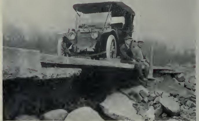
A severe test on the strength of lateral bonds in grouted brick pavement.
